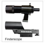
**Finderscope:** A finderscope is a small auxiliary telescope, attached to and aligned with the main telescope. It has low power magnification, a wide field of view and a crosshair to aid in centre. It can help you in finding and aiming at objects which you are intended to observe through the main telescope. Most finderscopes give an upside down or left-right reverse image.
