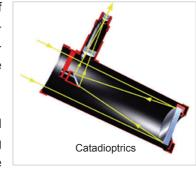
magnification of the correcting lens. In other words, if the correcting lens produces a 2x magnification and the physical length of the system is 500mm, the focal length becomes 1000mm. This design is very portable, being lighter and more compact than a normal Newtonian of the same focal length. It is easy to set up and aim and is much less subject to wind vibration. The correcting lens is factory aligned and the mirrors are user collimated like a regular Newtonian.
