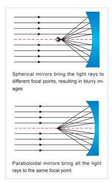
To overcome this defect, mirror surfaces are shaped during polishing to a paraboloidal shape which focuses all of the light rays to the same point.
