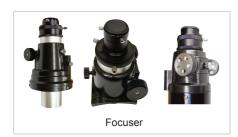
**Focuser:** The focus assembly is a device to bring the image into sharp focus. It usually moves the eyepiece back and forth with a rack-and-pinion or with a screw-in assembly. It should move smoothly and the image should not jump around as it is adjusted. Standard focusers accommodate eyepieces with 1.25 inch diameter barrels although 2 inch are also becoming more common.
